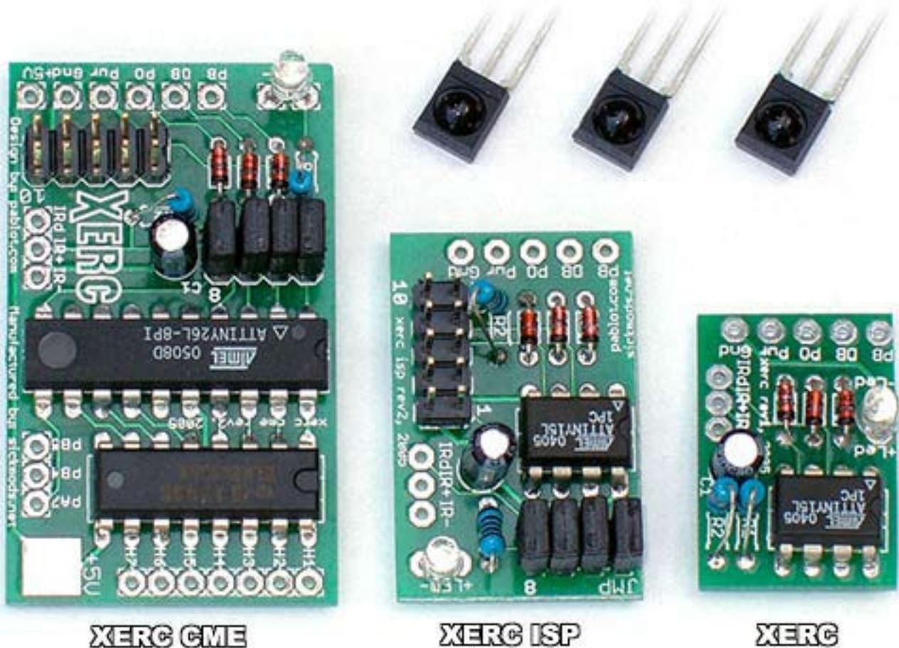
XERC is the simple version offering On/Off, eject, and modchip functions if your modchip supports it. Works on all Xbox versions. The ISP version is completely re-programmable, while installed in the Xbox (programmer not included).
