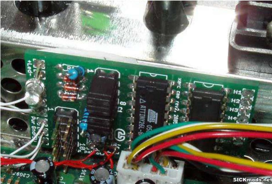
This is another example on how to place the XERC CME P12. Be sure to insulate it properly. It is held in place with hot-glue. The yellow wire coming from the back is for the VU-meter and the green wire from the DuoX 2 is for the BT points that the DuoX 2 needs.
