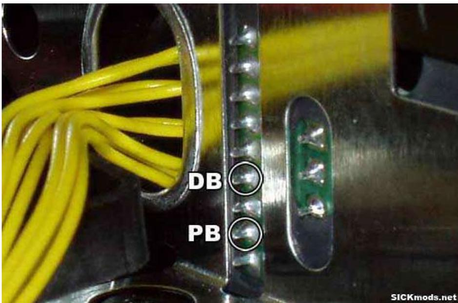
The PB and DB can be wired straight to the back of the power/eject PCB in the face of the Xbox. Refer to the following diagram:
